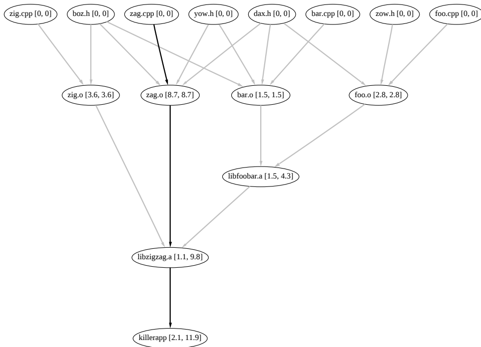
Figure 3.4 For each vertex there are two numbers: compile cost and accumulated compile time. The critical path consists of black lines.
