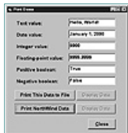
Figure 15.14. The frmPrint form demonstrates how to use the Print statement to output text data in a variety of formats.
