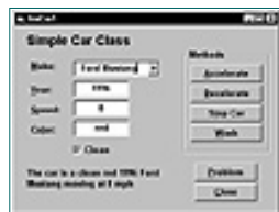
Figure 10.3. The frmCar1 form creates an object from clsCar1 and provides an interface to its properties and methods.
