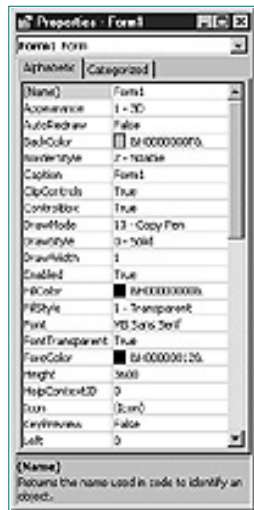
Figure 5.7. The Properties window contains most of the property settings for the object selected in the Form Designer window.
