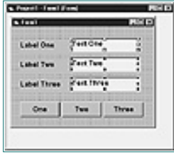
Figure 6.4. All the selected controls display sizing handles in their corners and along their edges.
