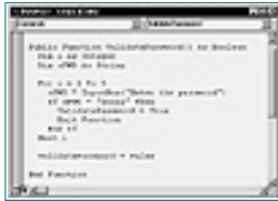
Figure 3.35. The upper limit of a For...Next loop can be hard-coded or set at runtime.
