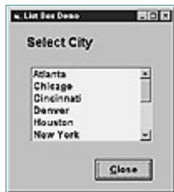
Figure 6.6. A list box is a handy way to present the user with a number of alternative values.
