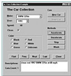
Figure 12.3. The frmCars form in the Cars.vbp project implements a Collection object to store car objects.
