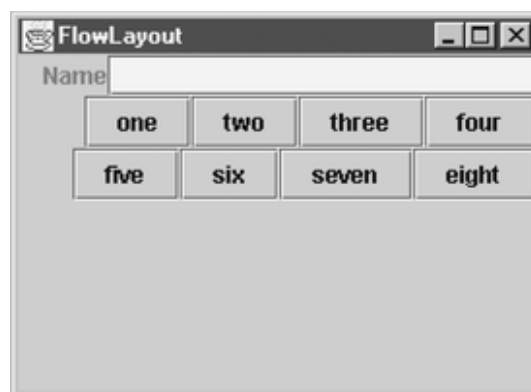
Figure 14-11. Vertical and Horizontal Gap Set to 0
