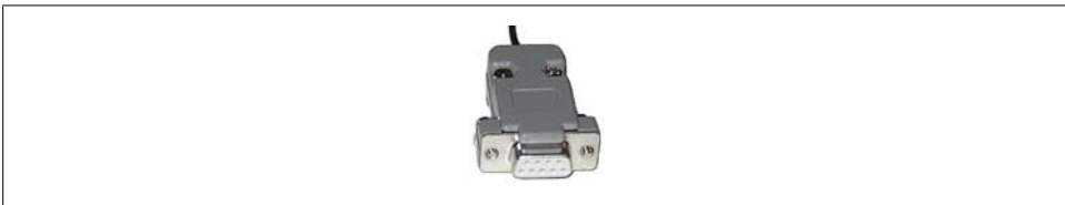
Figure 7-6. DB-9 connector with backshell assembly
